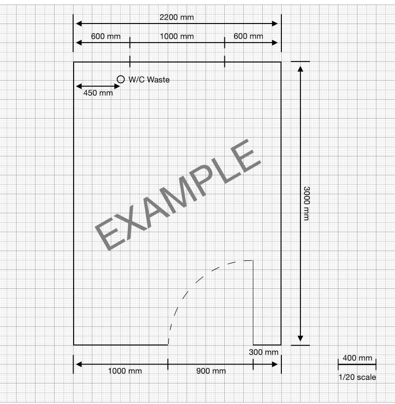
Please complete all room dimensions to include size of window and exact position, size of door including architrave and exact position and the position to the centre of the toilet waste.
